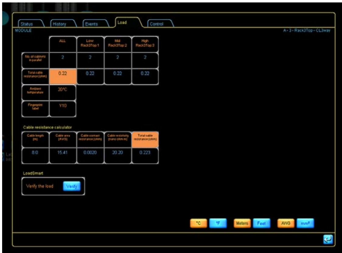
Figure 5.4: Load tab and LoadSmart Verification section
