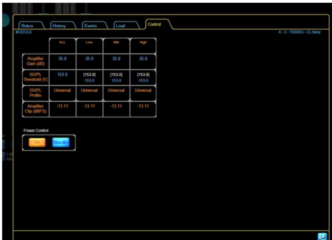
Figure 5-3: Control tab with parameters and power control
