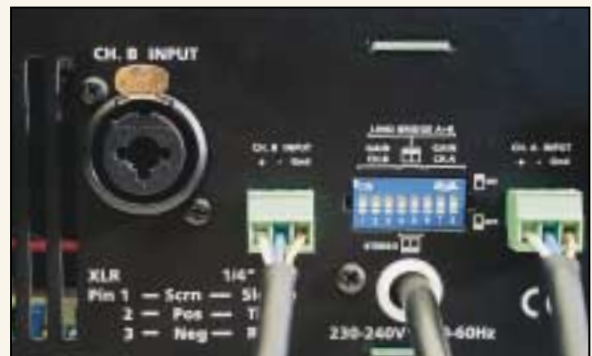
Neutrik Combo® input jacks adapt to both worlds, XLR or 1/4" phone plugs.
