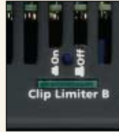
Recessed bypass switch per channel for the clip limiter.
