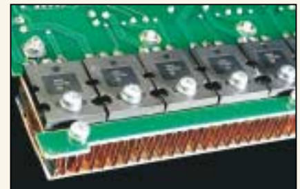
The output transistors are located side-by-side in the airstream
