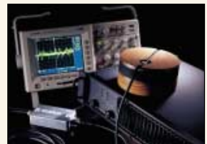
The very finest test equipment is made in-house; here is a coil for measuring the hum field.
